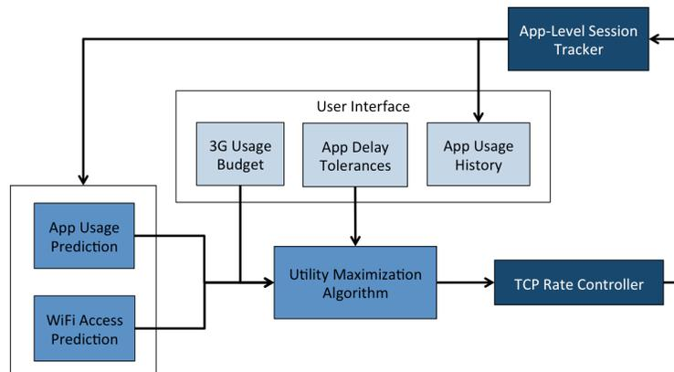
Figure 4: System modules and interaction across various components of AMUSE.
