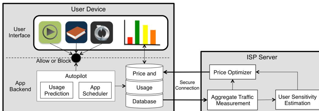
Figure 1b: Functionality separation between the user-side and operator-side devices.
