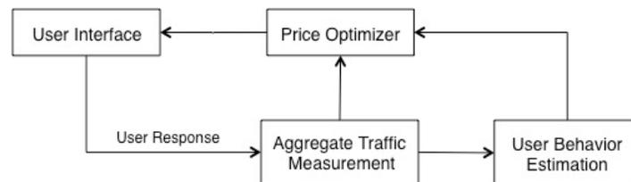
Figure 1a: Control-feedback loop of dynamic time-dependent pricing.
